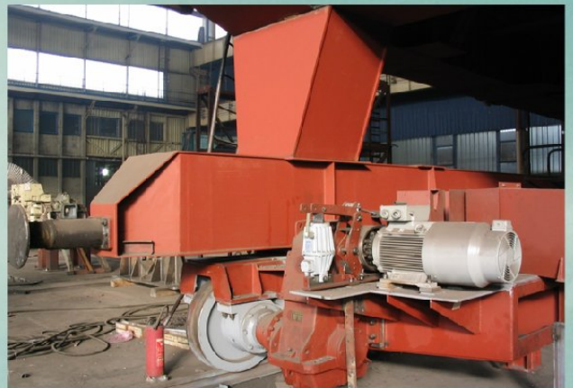
Installation of the electrohydraulic thruster in the Caterpillar excavator driver on surface mining Drmno, Thermal Power Station Kostolac
