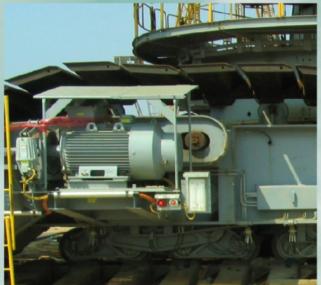
Electrohydraulic thruster embedded in the drive station on surface mining Drmno, Thermal Power Station Kostolac
