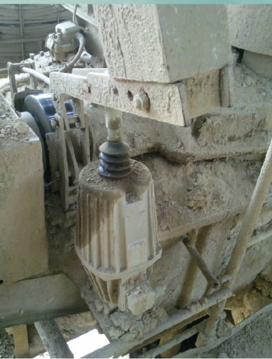
Electrohydraulic thruster built in on caterpillar drive in the RB Kolubara mine-Tamnava Zapad
